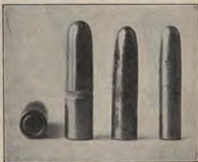
1 2 3 4 Fig. 104.—1, End view of 2, the Krag-Jorgensen bullet; 3, Mauser bullet; 4, Lee-Metford bullet, used by the United States Navy.
